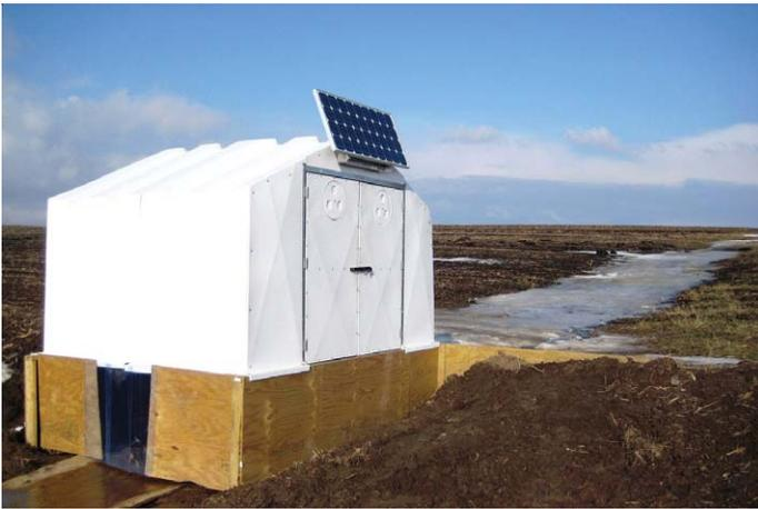
**Figure 3.** The enclosures installed at Pioneer Farm protect equipment (H-flumes, electronic samplers, data loggers) and help retain heat from propane heaters to keep gauges ice-free for improved data and sample collection.
