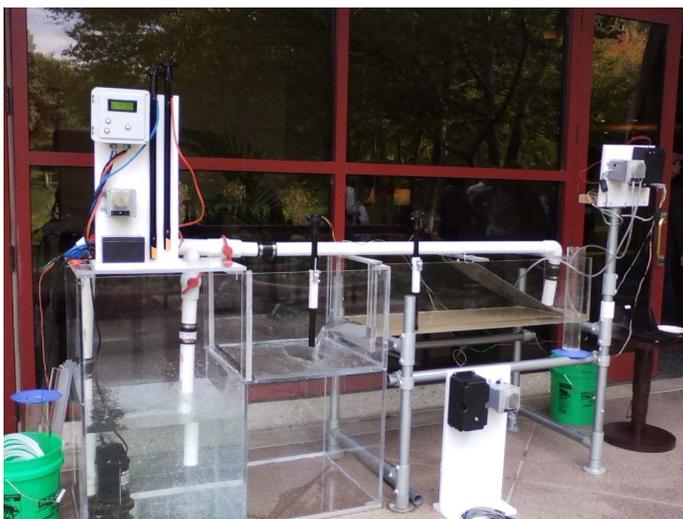
**Figure 1.** Recirculating flume set-up to demonstrate components of the prototype edge-of-field monitoring gauge.
