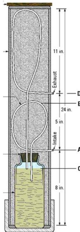
**Figure 2.** Construction of a single-stage siphon sampler (Credit: USGS Fact Sheet FS-067-00, May 2000)
